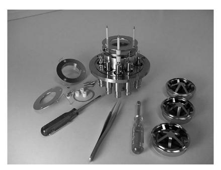
5. Remove Spacer and channel plate.
