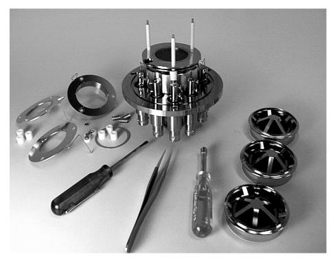
8. Disconnect lead from D2 barrel connector. Remove suppression grid and hold down plates being careful not to damage grid.
