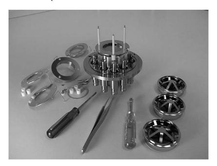
10. Take a new channel plate from its shipping container being careful to handle it by the outer rim. Blow off any dust with dry nitrogen or clean, dry compressed air. Do not use canned Freon. Do not allow anything to contact active area on microchannel plate as this will cause plate to be noisy.
