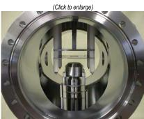
C-1551 Solid Sample Probe and Load Lock Assy C-1570 MALDI High Voltage Source Mounted on RETOF
